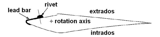
The bars must have a maximum width of 15mm and a maximum thickness of 1.6mm.
